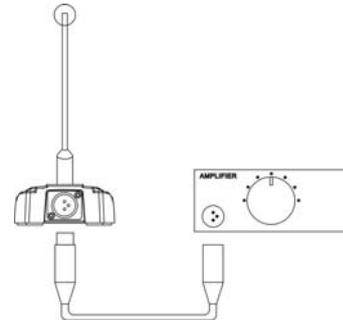
3. Microphone detachment: Press the release tab of the XLR socket on the microphone stand and pull out the microphone.
