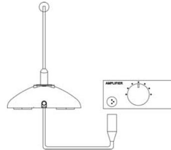
3. Microphone detachment: Press the release tab of the XLR socket on the microphone stand and pull out the microphone.
