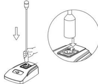
2. Connecting amplifier: Connecting 3-pin XLRM-type connector to other devices such as amplifier, audio mixing console, etc.
