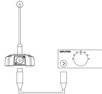
3. Microphone detachment: Press the release tab of the XLR socket on the microphone stand and pull out the microphone.
